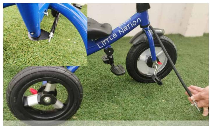
Ensure the parent steer rod bracket of the handlebars is on the same side of the trike as the parent steer on the parent handle. If this is not the case, loosen the handlebar clamp and turn the handlebars 180 degrees.
